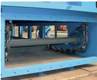
Figure 65: drive unit, tensioning unit division for SCC, using HEKO compo- nents
